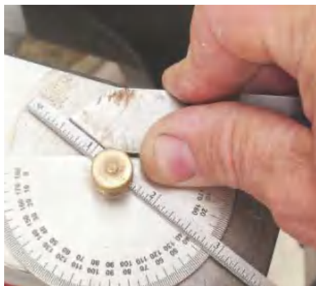
◀ Pic.3 40° is a good angle for the chisel. You need to apply a bit of strength at the business end of this tool
